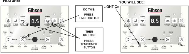
Note: For Delay Stop, the unit must be in the On position.
